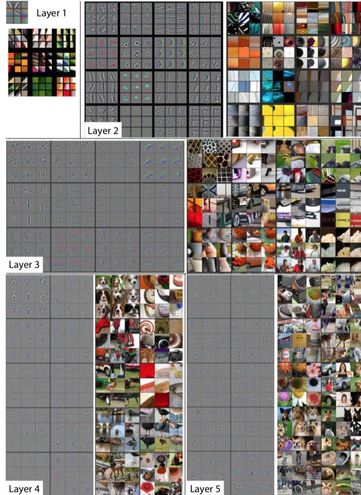
Figure 2. Visualization of features in a fully trained model. For layers 2-5 we show the top 9 activations in a random subset of feature maps across the validation data, projected down to pixel space using our deconvolutional network approach. Our reconstructions are not samples from the model: they are reconstructed patterns from the validation set that cause high activations in a given feature map. For each feature map we also show the corresponding image patches. Note: (i) the strong grouping within each feature map, (ii) greater invariance at higher layers and (iii) exaggeration of
