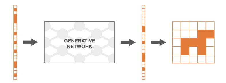
Input random variable (drawn from a simple distribution, for example uniform). The generative network transforms the simple random variable into a more complex one. Output random variable (should follow the targeted distribution, after training the generative network). The output of the generative network once reshaped.
