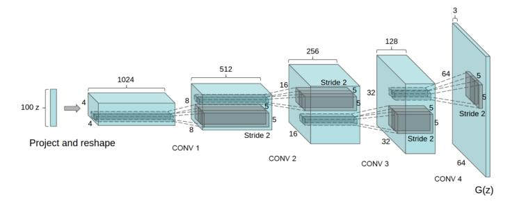
DCGAN generator used for LSUN scene modeling. A 100 dimensional uniform distribution Z is projected to a small spatial extent convolutional representation with many feature maps. A series of four fractionally-strided convolutions (in some recent papers, these are wrongly called deconvolutions) then convert this high level representation into a  $64 \times 64$  pixel image. Notably, no fully connected or pooling layers are used.
