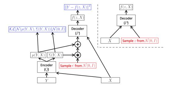
Left: a training-time conditional variational autoencoder implemented as a feedforward neural network, following the same notation as Figure 4. Right: the same model at test time, when we want to sample from P(Y|X).
