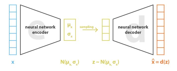
loss =  $||x - \hat{x}||^2 + KL[N(\mu_x, \sigma_x), N(0, I)] = ||x - d(z)||^2 + KL[N(\mu_x, \sigma_x), N(0, I)]$
